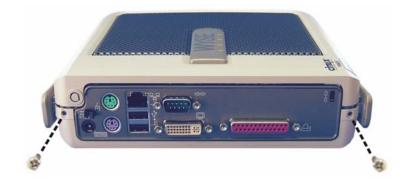
4. Remove the top cover from the thin client by inserting the tip of a small Flat-Edge Screwdriver just inside the edge of the lock receptacle to make contact with the metal liner that lines the opening. Apply pressure inward and downward on the metal liner while pulling up on the plastic housing until it releases.
